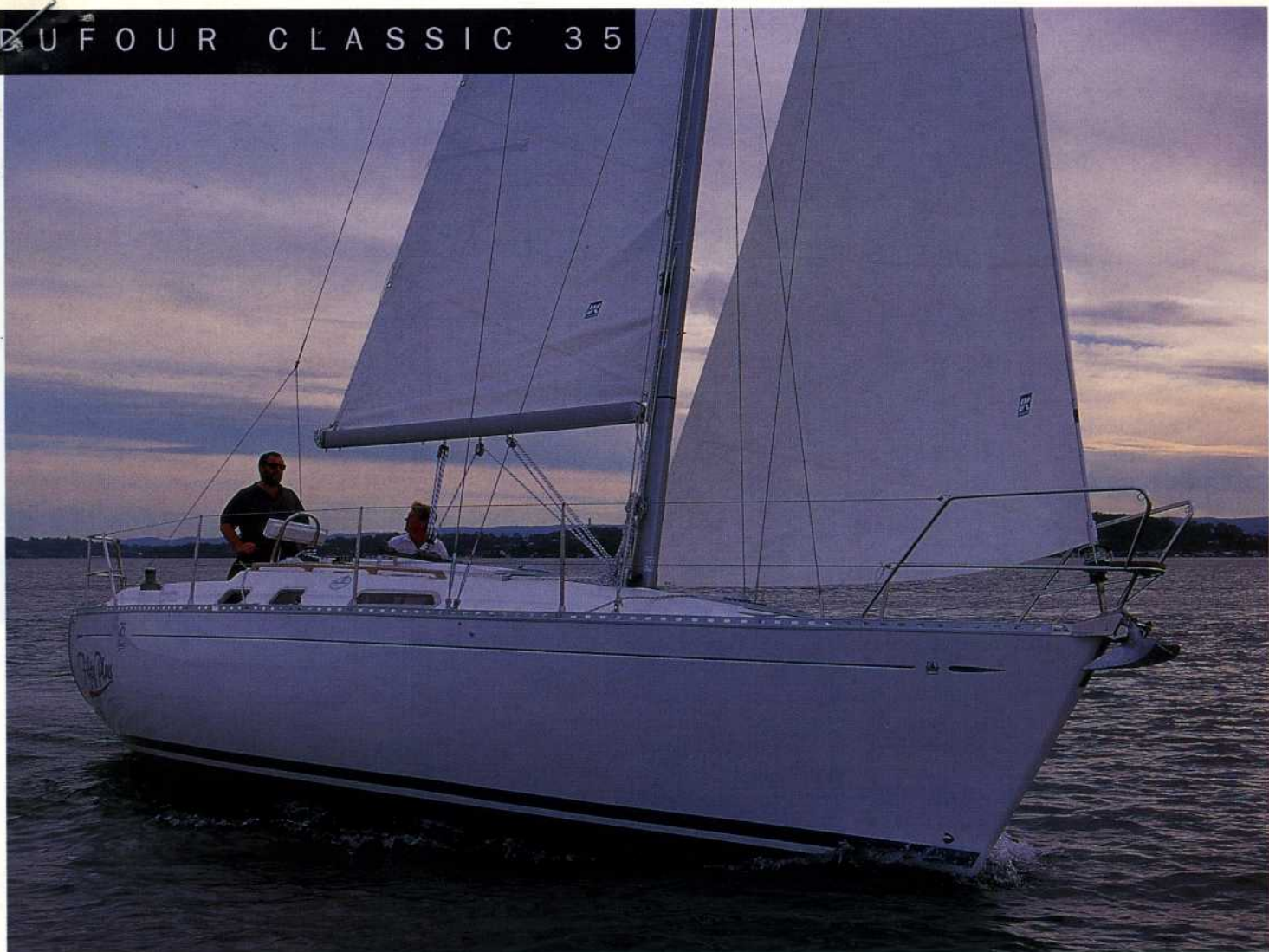
Hull lines are clean and moderate; headsail is set up on a roller furling system.
